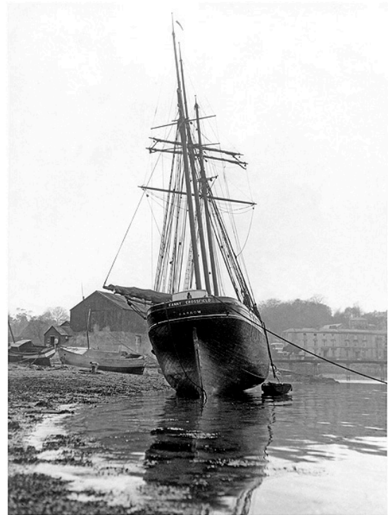
3-mast schooner FANNY CROSSFIELD 319 GRT, 55.6 x 22.5 x 9.0, built by Paul Rogers, Carrickfergus in 1880, the Strangford Lough 1938. Built for James Fisher & Son, Barrow, sold 1922 to Barrow of Penconer, her owners when seen here at Bar, Falmouth, on 11 April 1931. Falmouth motor quay just on beach - Mazon stowed to port, to keel vessel towards rising shore - Schmirler Pier & Emmer Place
